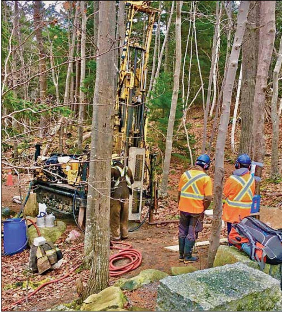
Geotechnical team investigated soil permeability and depth of bedrock next to the Williams Lake dam in the Shaw Wilderness Park PHOTO: CATHY VAUGHAN, DECEMBER 18, 2023
